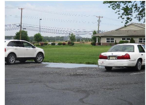
A rain garden can be installed to capture, treat, and infiltrate runoff and mitigate flooding in the northern parking lot. A preliminary soil assessment suggests that the soils have suitable drainage characteristics for green infrastructure.
