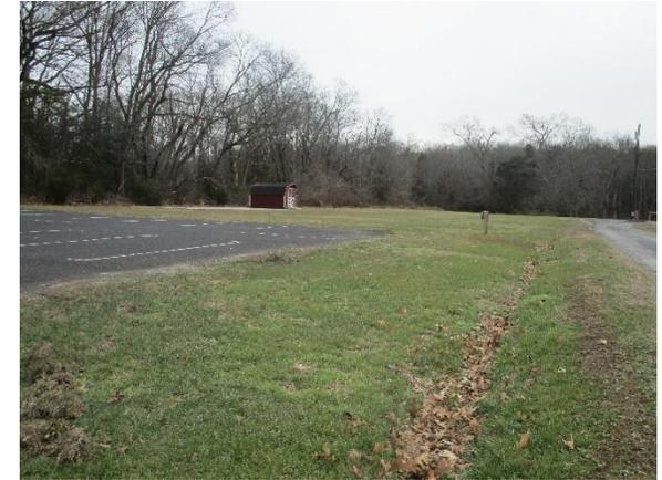
The existing swale can be converted into a bioswale, which would remove pollutants and convey water to the turfgrass area. Downspouts can be diverted into the bioswale as well. The parking lot is pitched toward the southwest, therefore the row of parking spaces furthest west in the parking lot can be replaced with porous asphalt to provide stormwater a chance to infiltrate. A preliminary soil assessment suggests that the soils have suitable drainage characteristics for green infrastructure.
