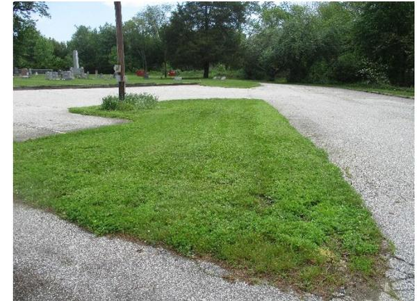
Parking spaces in the southwest corner of the parking lot can be replaced with pervious pavement to capture and infiltrate stormwater. A rain garden can be installed in the turfgrass island to capture, treat, and infiltrate runoff from the northern parking lot. A preliminary soil assessment suggests that the soils have suitable drainage characteristics for green infrastructure.
