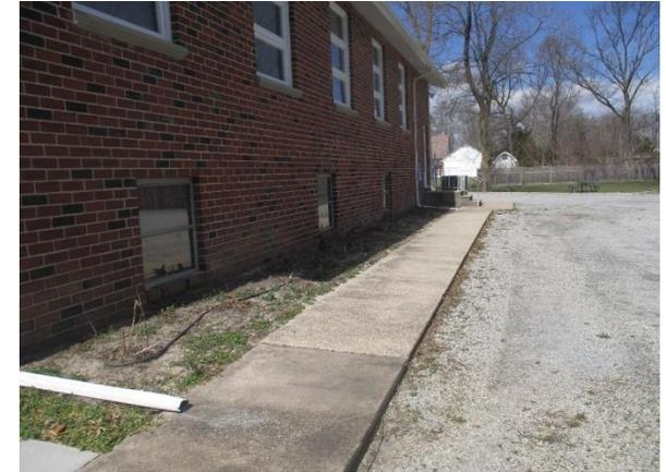
The parking lot is gravel, and the church has a basement. Downspout planter boxes can be constructed along the east and south side of the building to allow roof runoff to be reused. A preliminary soil assessment suggests that the soils have suitable drainage characteristics for green infrastructure.
